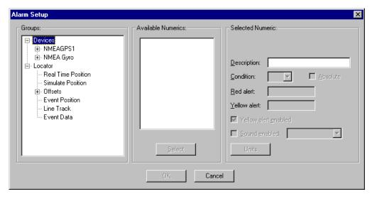
Click on the "+" symbol beside a **Device** or **Vehicle Name** to expand the list of items that can be added to the **Alarm** list. All items which can be selected for a particular **Vehicle** or **Device** are listed in the **Available Numerics** portion of the **Alarm Setup** window.
