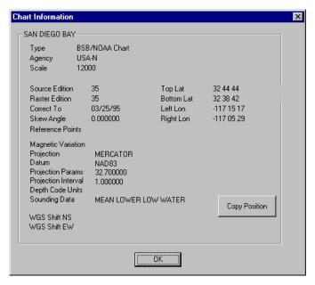
The **Chart Information** dialog box displays a variety of important details about the loaded NOAA Raster chart including the **Geodetic Datum** that the chart refers to, as well as to which **Sounding Data** the displayed **depths** refer.
