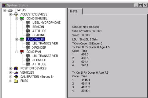
This node lists all the LBL and USBL acoustic devices that have been added to WinFrog. The devices are listed with an icon indicating the status of the serial port. Each device node can be expanded to list the data types associated with it.
