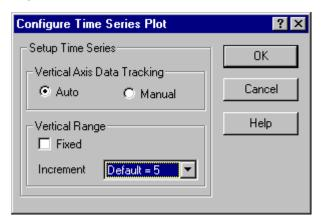
Use the **Configure Time Series Plot** dialog window to configure **Automatic** or **Manual** control of the **Vertical** (distance) **Axis** mid-point and the total range of the vertical data displayed.
