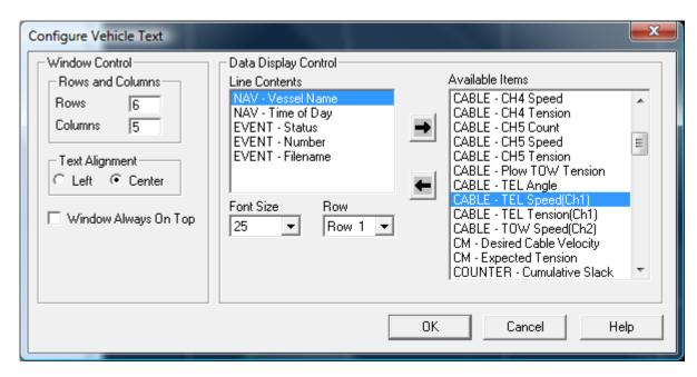
This window allows you to select which data items are displayed in the **Rows** and **Columns** of the **Vehicle Text** window, as well as the Font Size and Alignment of the selected data text.
