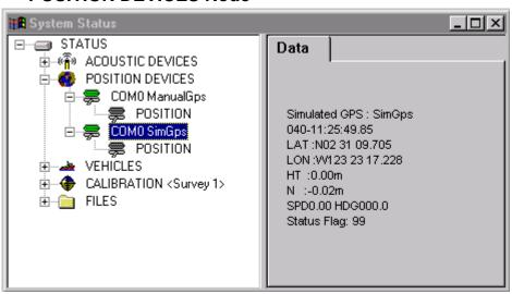
This node lists all the position type devices (GPS) that have been added to WinFrog. The devices are listed with an icon indicating the status of the serial port. Each device node can be expanded to list the data types associated with it.
