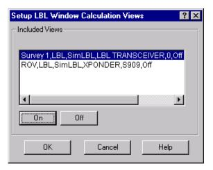
All data types available for viewing using the time series window are listed in the list box. They are given by vehicle name, device type, device name and data type name. Select one and click the **On** button. If you wish to view more than one, select another and click the **On** button again. Note that the window will become cluttered and difficult to interpret if too many data types are displayed. Click **OK** to exit this dialog and view the time series window.
