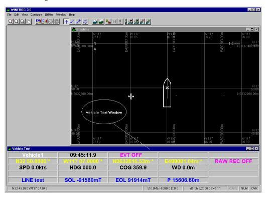
WinFrog carries a default configuration of the **Vehicle Text** window contents for the initial start up. The data displayed in this window (and the location of data items in the window) is configurable as detailed below. All modifications to the Vehicle Text window are saved in the **WinFrogini.wfg** file when the program is exited correctly.
