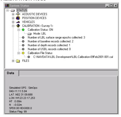
This node summarizes the calibration status for the vehicle selected for the calibration for the window (see **Select Vehicle for Calibration**). The primary node caption includes the name of the vehicle selected or None if one has not been selected.
