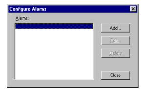
2 Click on the **Add** button to bring up the **Alarm Setup** window, as seen below.
