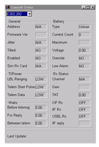
A dropdown list box at the top left of the window presents a list of the transponders available for viewing in this window. When selected, the extended status information is displayed in the appropriate read only boxes.
