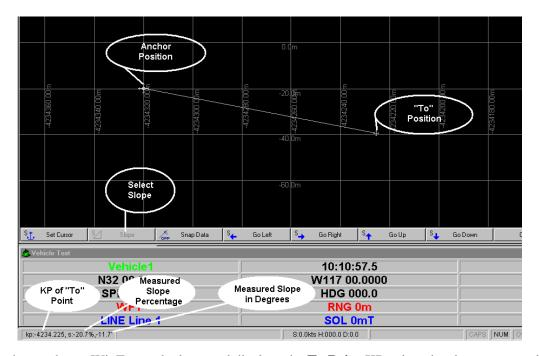
As shown above, WinFrog calculates and displays the **To Point** KP value, the slope measured in degrees, and the measured slope percentage.
