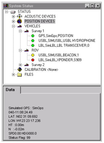
This node lists all the WinFrog vehicles that have an acoustic data type attached to them. These nodes can be expanded to list the POSITION, LBL and USBL data types attached to the respective vehicle. Note that only these data types are listed.
