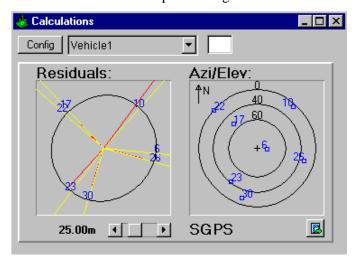
The azimuth and elevation of the GPS satellites used in the pseudorange solution are displayed too.
