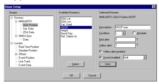
4 Type in a description for the device in the **Description** entry window.
