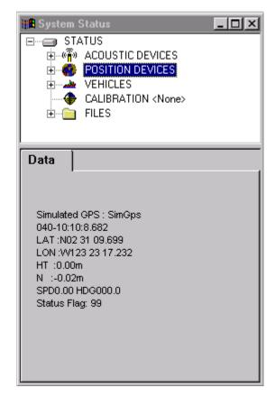
This split window presents the configuration of WinFrog in a tree format in one panel and data in the other panel. The split can be configured to vertical or horizontal via a pop-up menu using the right mouse button in the tree section. The font used in the data section can be modified via a pop-up menu using the right mouse button in the data section.
