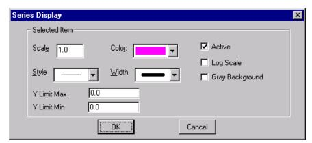
From this dialog, the line color and width can be selected. The plot for the respective data can also be enabled or disabled by checking or un-checking the **Active** checkbox. In addition, the background can be toggled between gray and white by checking or unchecking the **Gray Background** checkbox.
