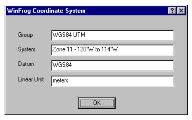
5 A **Map Coordinate System** dialog opens to configure the BML map file coordinate system. Set the BML file geodetics to the WinFrog geodetics from the previous step – this
