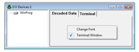
The I/O Devices window is divided into two sections: The left side of the window lists all devices that have been added to WinFrog, while the right side of the window displays **Decoded** Data and the Terminal tab if enabled.
