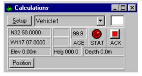
The selected vehicle's current **Latitude**, **Longitude**, **Elevation**, **Heading**, and **Water Depth** are updated every program cycle.
