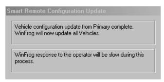
**Note:** The remote will accept a configuration update from any master. There should be only one master on the network at one time.
